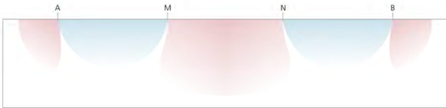
Figure 6. Schematic example of 2D-sensitivity distribution for a homogeneous half-space and a specific electrode geometry with current electrodes A and B and potential electrodes M and N. An increase of the parameter value in a positive area (pink) will increase the magnitude of the measured quantity, while the magnitude will decrease if the parameter increase takes place in a negative area (blue).
